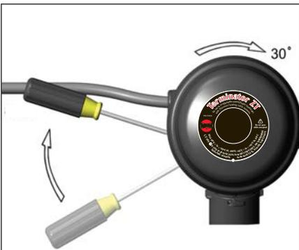
15. Use screwdriver to ratchet on junction box lid. Lid will rotate 30 degrees. To remove lid, repeat steps 14 and 15 but in the opposite direction.
