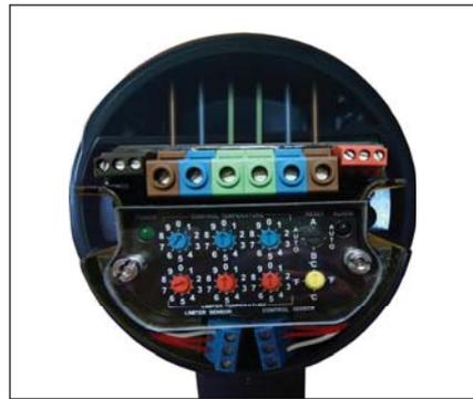
14. Install electronic control module and complete system wiring. Terminal set screws shall be tightened to a torque value of 1,4 Nm (12,4 lb-in). See page 5 for wiring details. Set modules electronic control and/or control limiter at desired setpoints.
