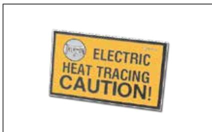
**CL...** vinyl-based peel-and-stick caution labels are intended for direct exposure to industrial environments. Electrically heated pipelines and vessels should be clearly identified at frequent intervals along the pipeline or vessel. Caution labels should be placed at 3 to 6-m intervals or as required by code or specification. Additional languages or other texts are available; contact Thermon.
