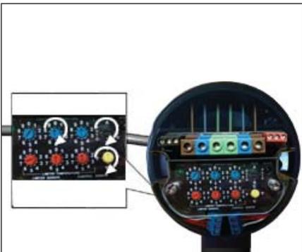
12. Use the rotary switches for settling Control and Limit Temperature, (Celsius or Fahrenheit) and Auto or Manual reset (Control switches on Type "C", Limiter switches on Type "L" and both on Type "CL").
