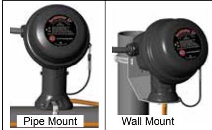
**Terminator ZP...** is designed to fabricate power connections, in-line/T-splice connections or for making end terminations. The Terminator ZP-XP is suitable for use in hazardous areas (Ex e T6/T4), harsh industrial environments and has a IP66 rating. The upfront positioning of the terminal block permits easy access during assembly and for future routine maintenance.
