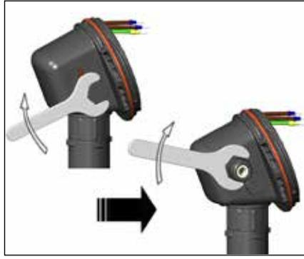
**10.** Remove M25 dust cap. Install M25 power gland (order separately) and M25 blind plug. For in-line splice, T-splice, or end termination, install additional M25 blind plug (order M25-B-EXE separately) instead of M25 power gland.
