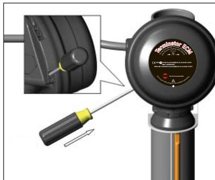
13. Install junction box lid and twist hand tight. Insert screwdriver into ratchet slots located on side of junction box base.
