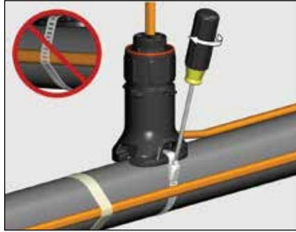
**Terminator:** Route cable through base entry and mount expediter to pipe using pipe band. Do not band over cable.
