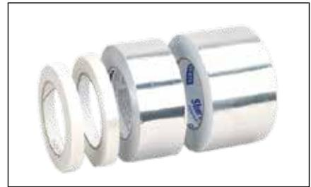
**FT-1L, FT-1H...** fixing tape for attaching heating cable to piping every 300 mm or as required by code or specification.
