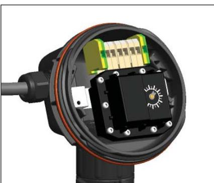
16. Install thermostat and complete system wiring. Terminal set screws shall be tightened to a torque value of 1.4 Nm (12.4 lb-in). See page 5 for wiring details. Set thermostat at desired setpoint.
