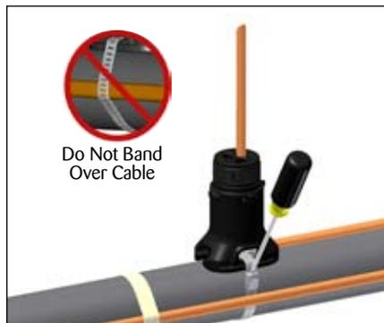
**5.** Mount expediter to pipe using pipe band. Do not band over cable.
