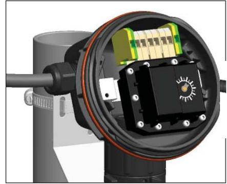
11. Install thermostat and complete system wiring. Terminal set screws shall be tightened to a torque value of 1.4 Nm (12.4 lb-in). See Step 13 for wiring details. Set thermostat at desired setpoint.
