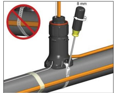
6. Mount expediter to pipe using pipe band. Do not band over cable.
