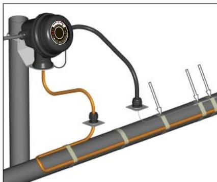
16. Fix thermostat bulb and capillary tube to pipe.
