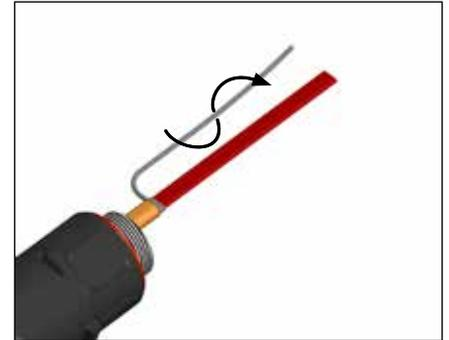
**1c.** Twist braid into a pigtail. Trim ends of braid.
