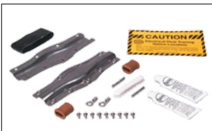
**SK-SX-OJ...** Ex e approved under-the-insulation repair and splice kit for overjacketed SX cables. Kit includes stainless steel shells, screws, grommets, RTV adhesive/sealant, insulation tape and the necessary wire pins/lugs.
