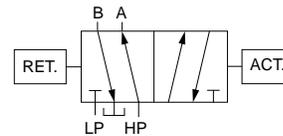
**3 POSITION 5/3** Diagrams below show center position only. Offset positions are same as shown above for 2-position types. To indicate particular center pattern required, substitute number shown within corresponding diagram for fourth digit of product number.
