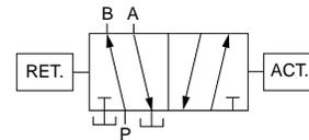
**3 POSITION 5/3** Diagrams below show center position only. Offset positions are same as shown above for 2-position types. To indicate particular center pattern required, substitute number shown within corresponding diagram for fourth digit of product number.
