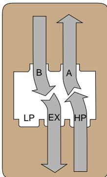
HP inlet open to cylinder port A;
