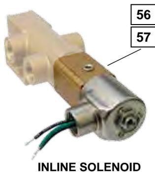
**INPilot-** utilizes the pressure from the inlet of the valve, through internal passages, to the solenoid-pilot. In this type valve, only one pressure connection, the inlet, is necessary.
