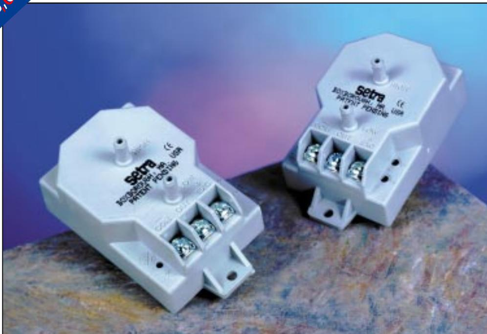
Setra Systems 265 pressure transducers sense differential or gauge (static) pressures and convert this pressure difference to a proportional electrical output. The 265 is offered with a high level 0-5 VDC output or a 4-20 mA output. It is also offered with 0-5 or 0-10 VDC output in the 24 VAC excitation version.
