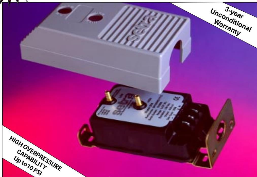
Setra Systems 264 pressure transducers sense differential or gauge (static) pressure and convert this pressure difference to a proportional electrical output for either unidirectional or bidirectional pressure ranges. The 264 Series is offered with a high level analog 0 to 5 VDC or 4 to 20 mA output.
