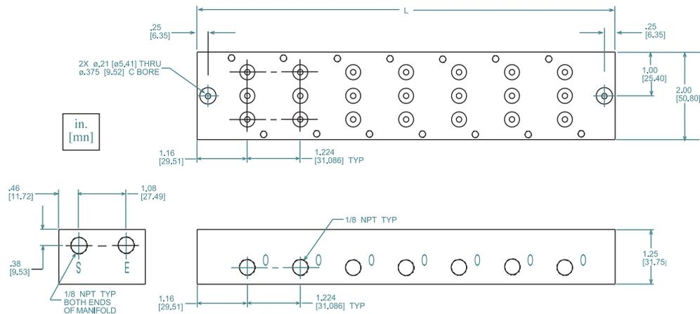
Manifolds are available in 2 to 10 stations. To calculate the overall length "L" of the manifold use the following formula:
